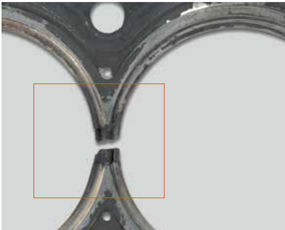
▲ Broken web caused by high component dynamics
