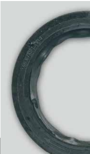
▲ Damaged PTFE sealing lip as the cause of failure.
