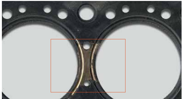
▲ Scorched elastomer coating
