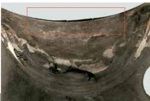
▲ Damaged gasket in the Ricardo squish area due to detached swirl chamber. Spacer sheet fractured in two places and pressed out.
