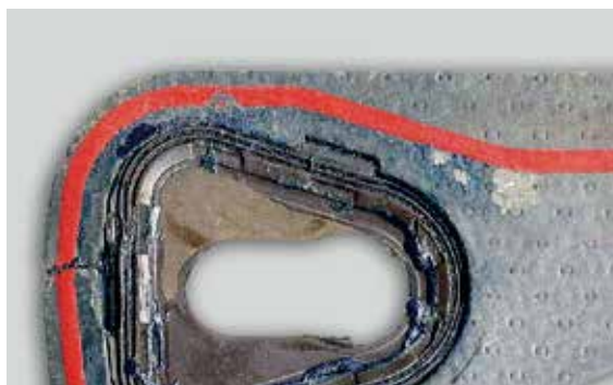
▲ Tearing and breakage of the composite material, and damaged Viton element due to incorrect application of additional sealing compound.
