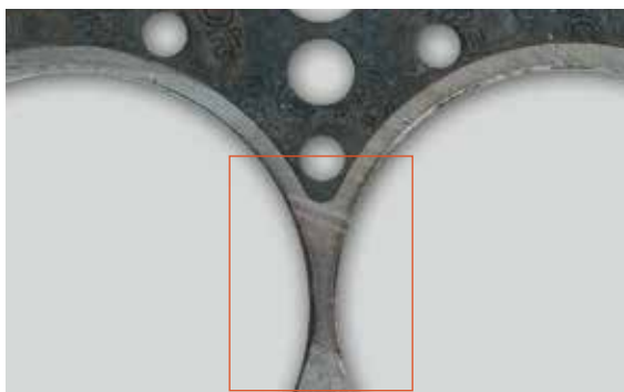
▲ Roughness of engine block and cylinder-head surfaces leads to gas blowby between the combustion chambers.
