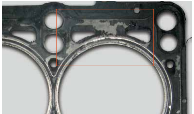
▲ Elastomer coating damaged by overheating
